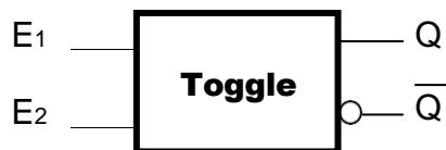
The flip-flop is the most common storage circuit. It also serves to create a frequency divider by two. It is a sequential system consisting of one or two inputs and two complementary outputs.
