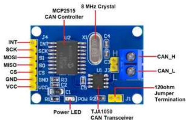
Figure 26. Pinout du Module CAN MCP2515
