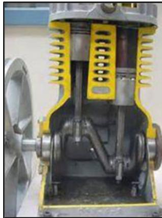
**Fig. II.1.** Piston compressor
