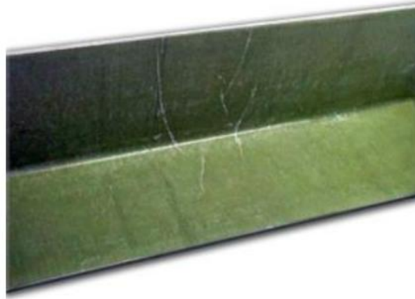
Figure IV. 15 : Defect with chipping.
