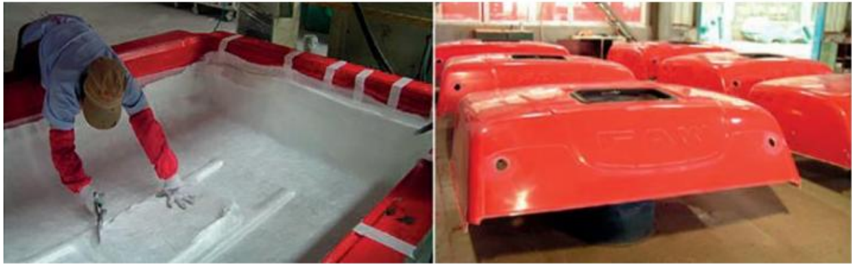
Figure IV. 7 : Low-Pressure Cold Compression Molding (Wet Method).
