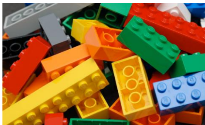
Figure. I.3: Part made of amorphous Acrylonitrile Butadiene Styrene (ABS) polymethyl methacrylate.
